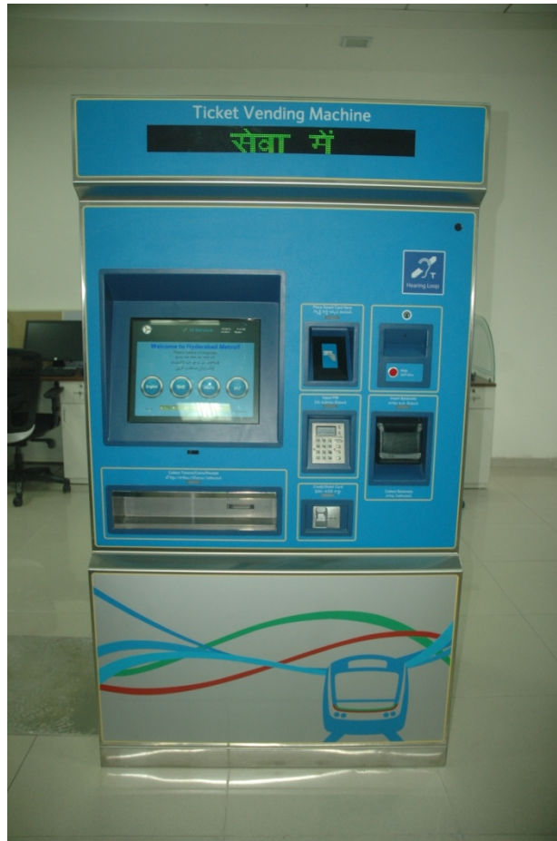
Ticket Vending Machine (TVM) at stations with different payment modes, such as Cash, Credit/Debit Cards etc.
